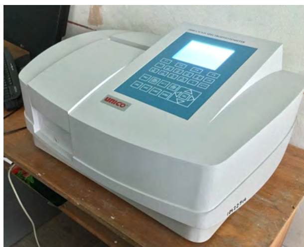
Fig. 2. Spectrophotometer UNICO 2800 used for spectral analysis of combustion residue extracts
