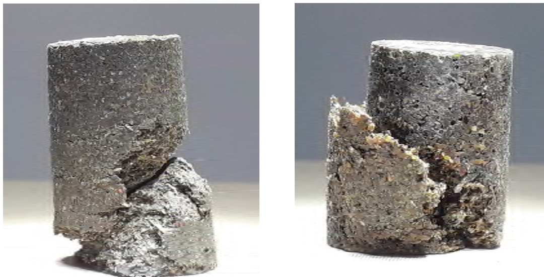
Fig. 6. General appearance of epoxy composite samples after compression with filler content (fraction less than 0.5 mm): a – 150 wt. parts; b – 200 wt. parts.
