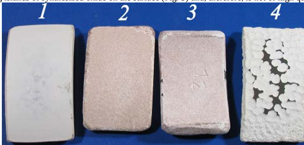
Fig. 3. Oxide-ceramic coatings on zirconium alloy (processing modes are given in Table 1)
