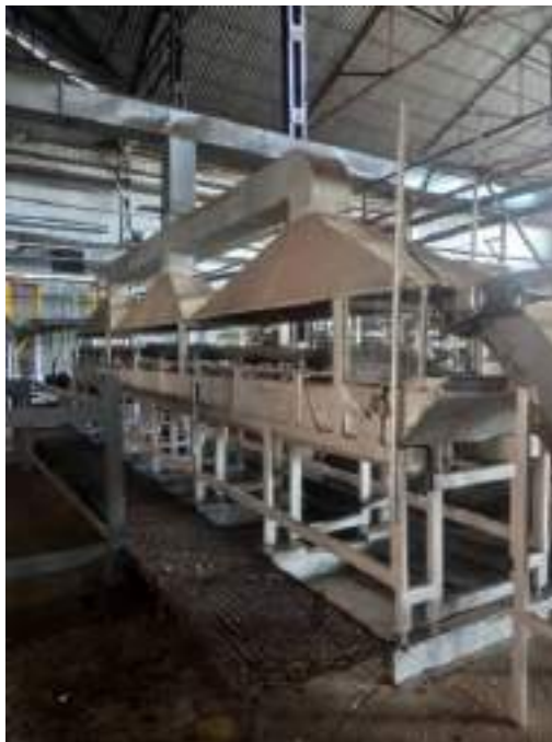
Fig. 2. Improved oven for roasting onions at the ChVZ LLC “Vidzi Production” of the Veres Group
