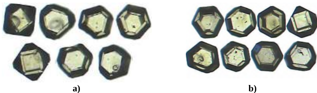
Fig. 2. Micrographs of diamond crystals of the AC250 brand with grain sizes: 630/500 (a) and 500/400 (b).
