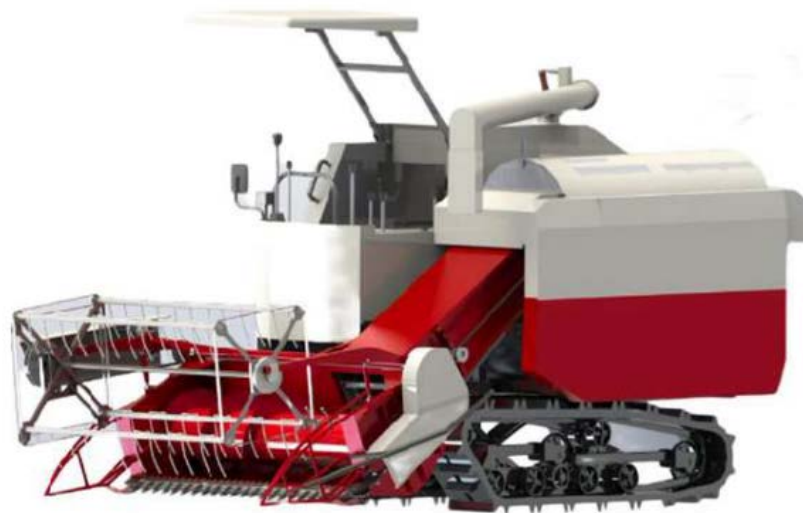
Fig. 3. Example of a modern tracked-type flax harvester developed in China, equipped with guiding elements that perform divider functions. Illustration provided by source [9] and manufacturer open-access materials
