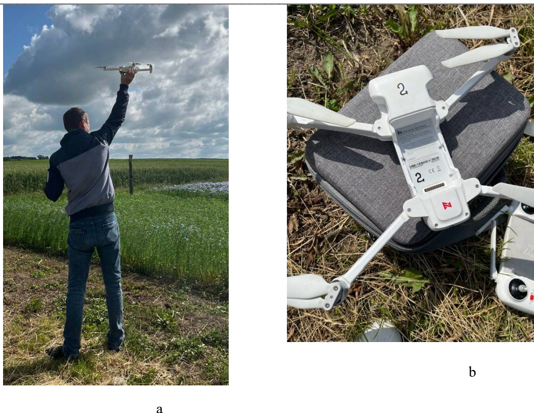
Fig 1. A UAV (drone) flying over an agricultural field to capture multispectral images: a – UAV launch; b – UAV used in experiments
