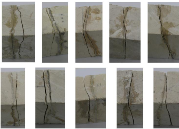
Fig. 4. Polymer-joined samples broken by three point bending test
