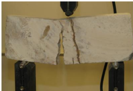
Fig. 6. Three point bending test of samples joined with epoxy mortar.
