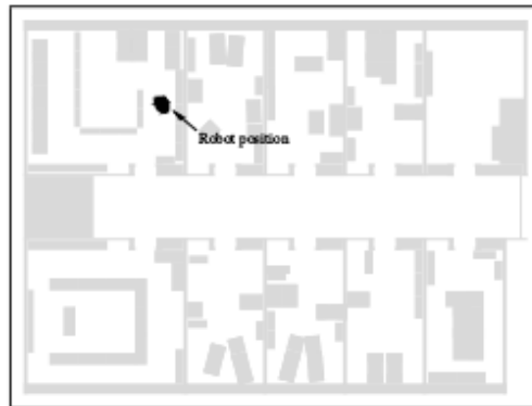
Fig. 4. - Robot's pose estimation by AMCL – after calculating [4].
