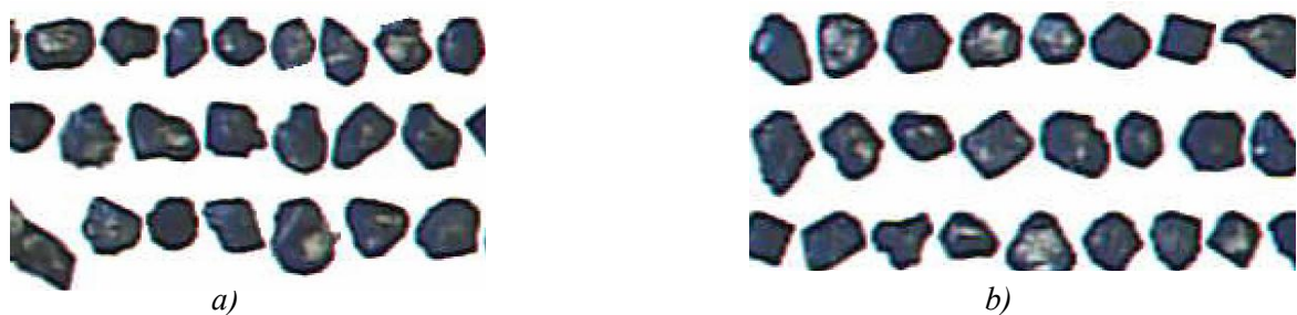
Fig. 1. Samples of AC20 100/80 powder before (a) and after HVED treatment, chemical cleaning and powder production (b)
