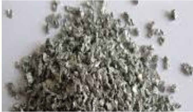
Fig. 1. - Overview of alloy AK12MMgN powder wastes microparticles after regeneration (on plastic plate), ×32
