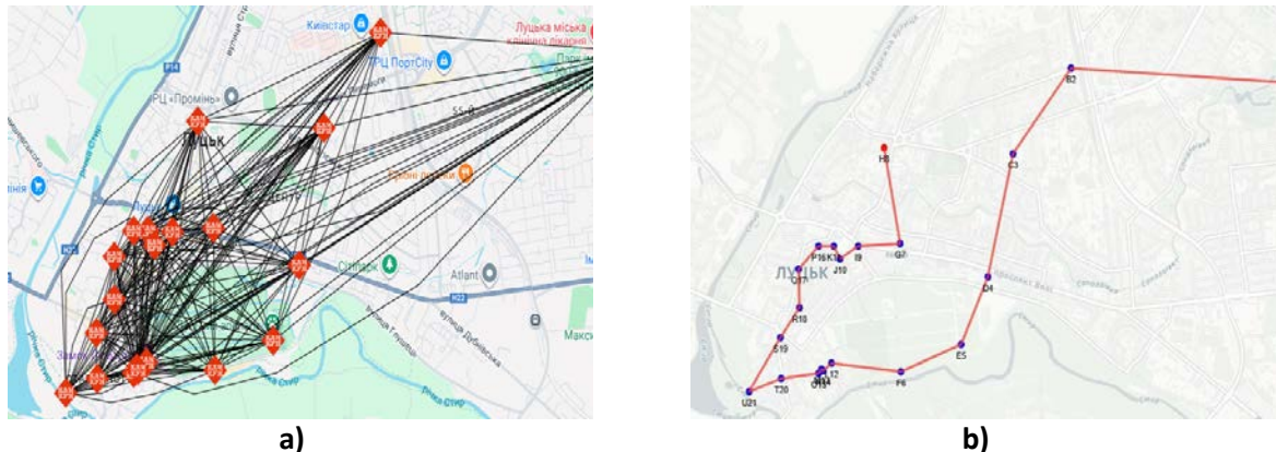
Fig. 4. Graph model of connections between tourist objects and the optimized pedestrian route obtained using the Greedy + 2-opt algorithm.
