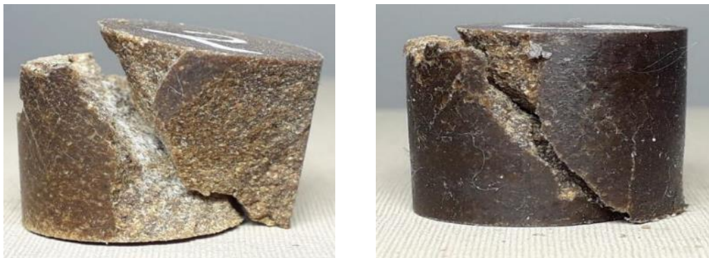
Fig. 3. The general appearance of biocomposite samples (with removal of 10% of moisture from the composition) after destruction with content of drying oil Oksol : a – 2 parts by weight.; b – 10 parts by weight
