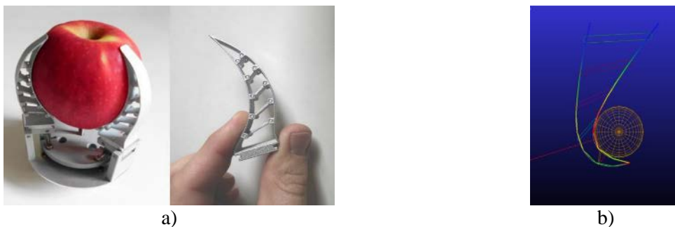
Fig. 6. Adaptive gripping device, a – working prototype, b – ADAMS model
