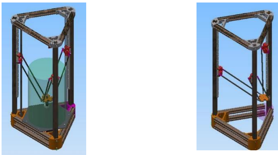
Fig. 1. Triglidge-based 3D printer model before and after simplification
