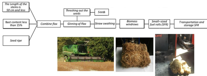
Fig. 2 – Technology of the flax stem primary processing, when length and bast content of the flax stems are not sufficient to obtain fiber of a proper quality
