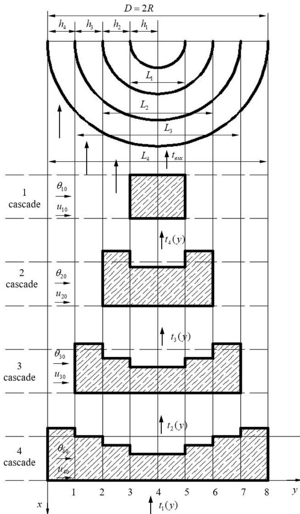
Fig. 3 – Calculation diagram of «cascade» drying at  $n = 4$
