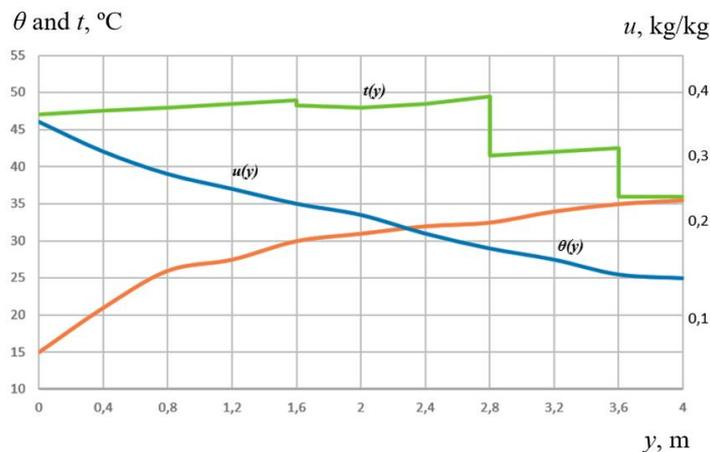
Fig. 4 – Results of the calculation of moisture content  $u(y)$ , seed temperature  $\theta(y)$  and drying agent temperature  $t(y)$
