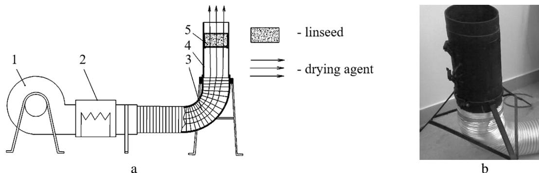
**Fig. 1** – Experimental equipment for linseed drying:
