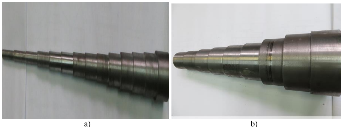
Fig. 5 Experimental specimens of steel 20 for determining the correction factor: a) sample diameter from 12 to 64 mm, b) sample diameter from 70 to 170 mm
