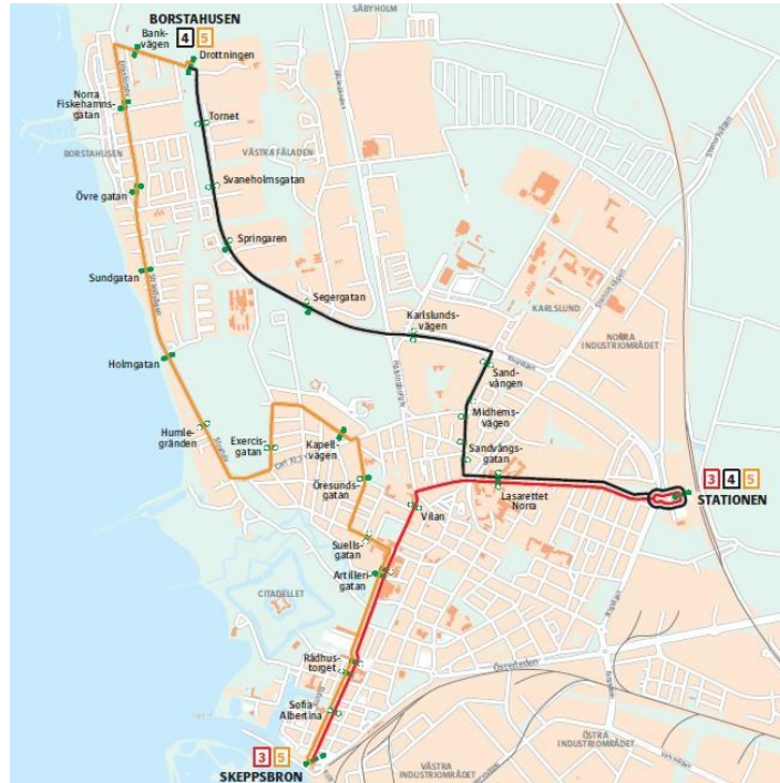
Fig/ 8. Trolleybus system in Landskrona, linie 3 - standard trolleybus line, lines 4 and 5 - battery operation [14]
