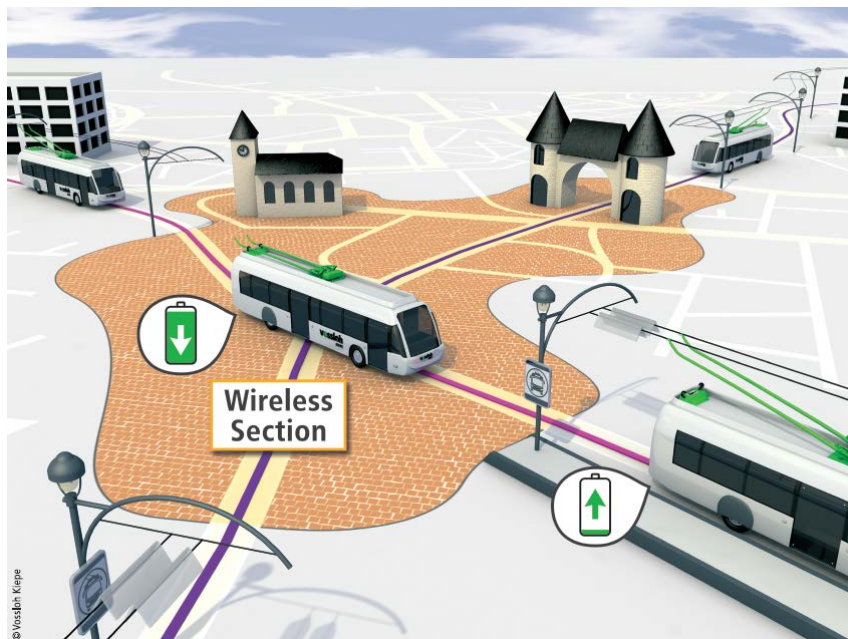
Fig.1. The idea of In Motion Charging system (IMC) [© Vossloh Kiepel]
