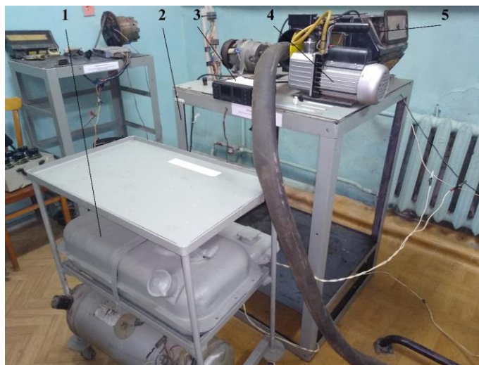
1 – air heating unit; 2 – stand frame; 3 – control panel; 4 – gas cooler damper control compressor; 5 – gas cooler-evaporator;
