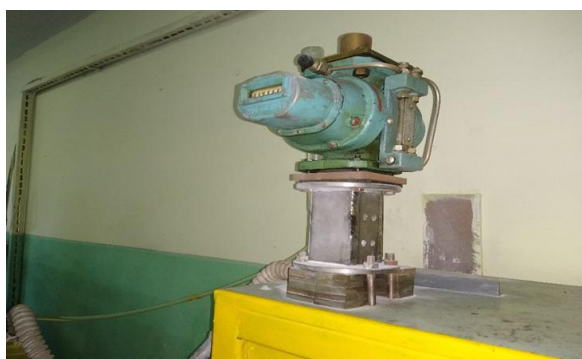
Fig. 4. Flowmeter for measuring volumetric flow of compressed gas
