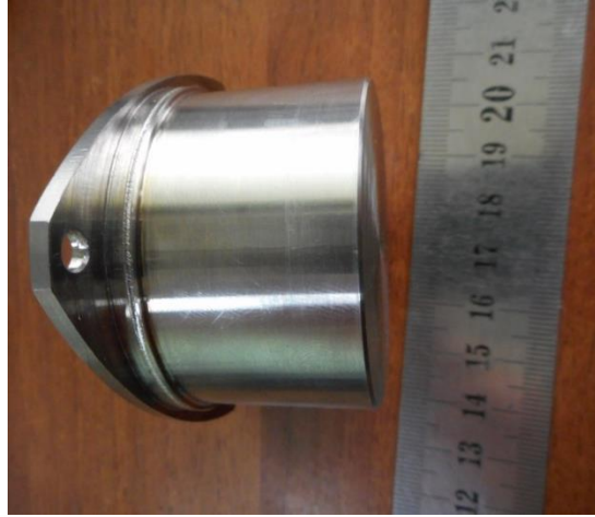
Fig. 8. Welded sensor part using the “cover with flanging” scheme
