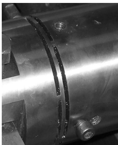
Fig.4. Machined spring of cross slot configuration of the toolholder (a) and experimental polar diagram of the flexibility of the elastic part of the toolholder (b)
