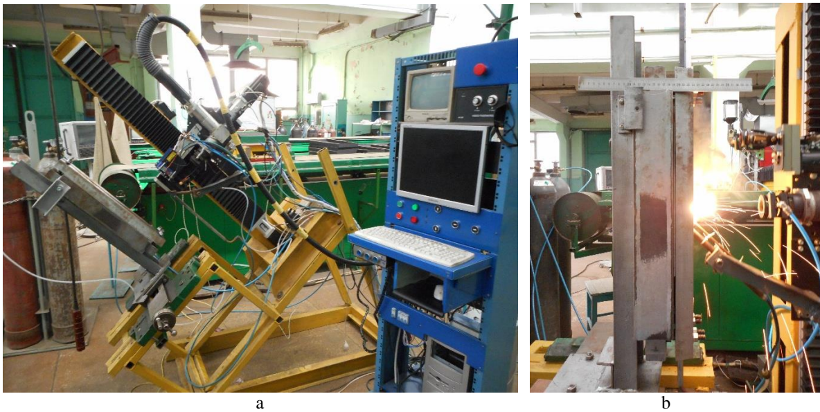
Fig. 4. Laboratory setup for laser welding in various spatial orientations (a); (b) the process of welding T-joints
