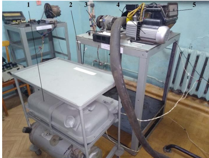
1 – air heating unit; 2 – stand frame; 3 – control panel; 4 – gas cooler damper control compressor; 5 – gas cooler-evaporator;
