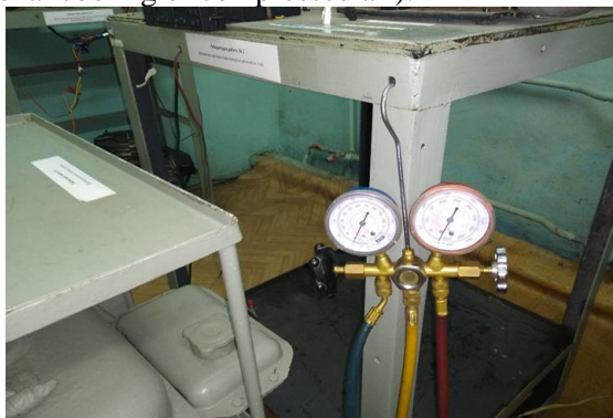
Fig. 3. Manometric manifold for measuring the compressed gas pressure of the installation
