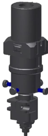
Fig. 3. 3D model of the optical head for laser welding
