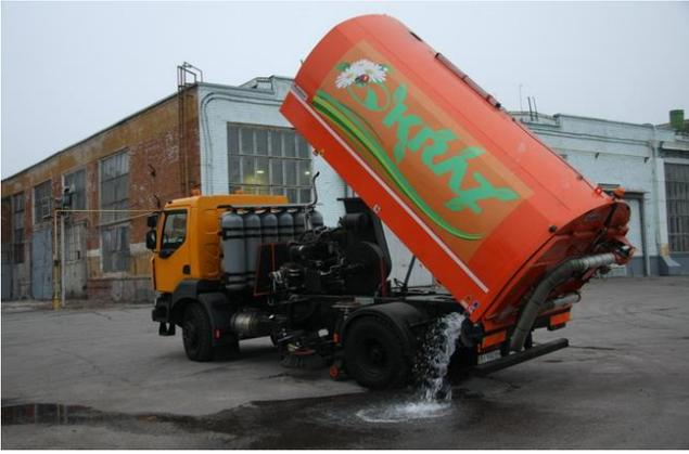
Figure 2 – KrAZ-5401K2 car with gas cylinder equipment
