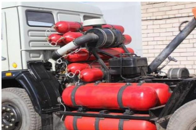
Figure 1 - Gas cylinder system of the MAN TGA 440PG car
