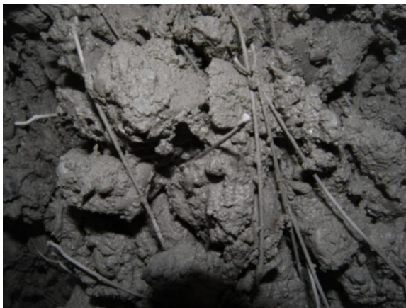
Fig 3. Steel fibers in concrete mixture
