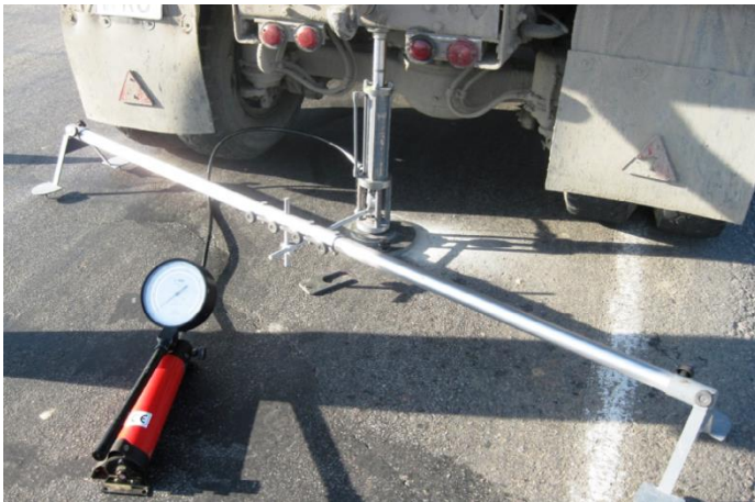
Fig. 1. Type of testing of pavement by stamping method device 35-T0116 / C "CONTROLS"
