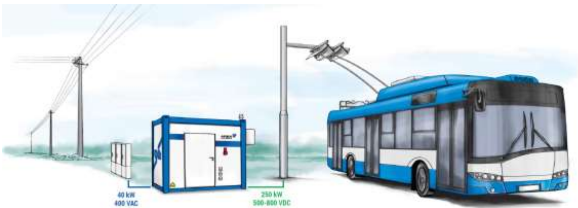
Fig. 6 – Stationary trolleybus charging station with energy storage (Firma AREX, Gdynia, Polen).
