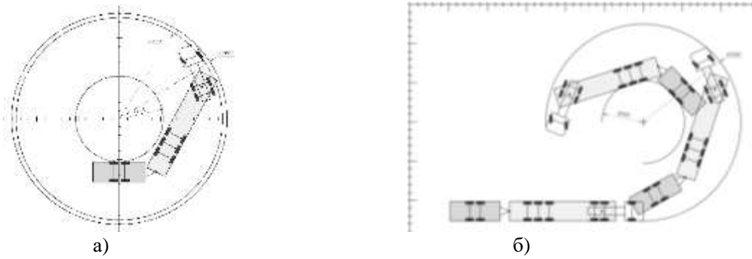
Figure 3. The dimensional traffic lane of a saddle-coupled three-link road train at circular motion (a) and entering a turn (b)
