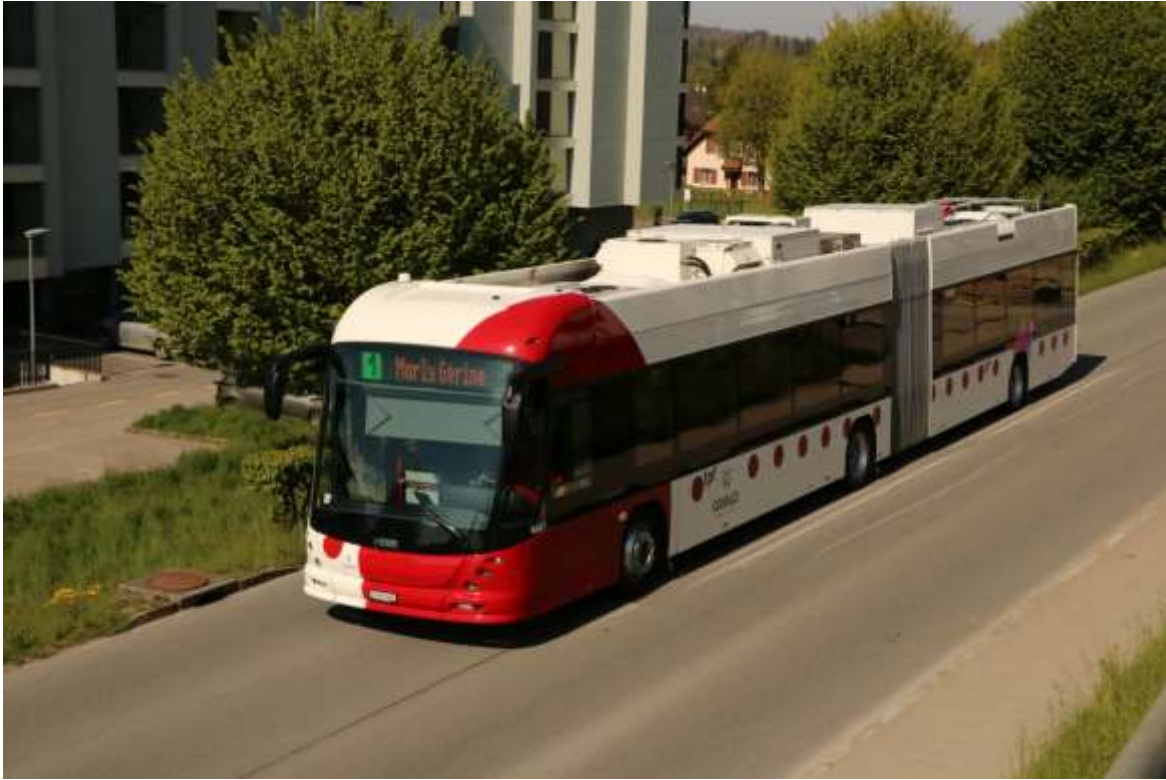
Fig. 11 – Hess light Tram 19 DC trolleybus on line 1 in Freiburg (Switzerland) with the dynamic charging system IMC. The route is only 30% covered by the trolleybus network and a 66 kWh LTO traction battery can be seen on the roof of the first vehicle section. Foto Mikołaj Bartłomiejczyk
