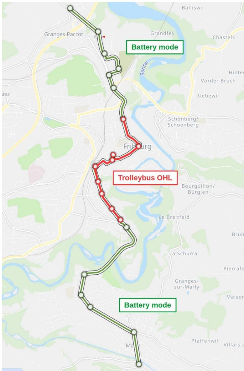
Fig. 10 – Line 1 in Freiburg, Switzerland, operated by IMC trolleybuses, only 30% covered by overhead catenary, based on https://moovitapp.com/
