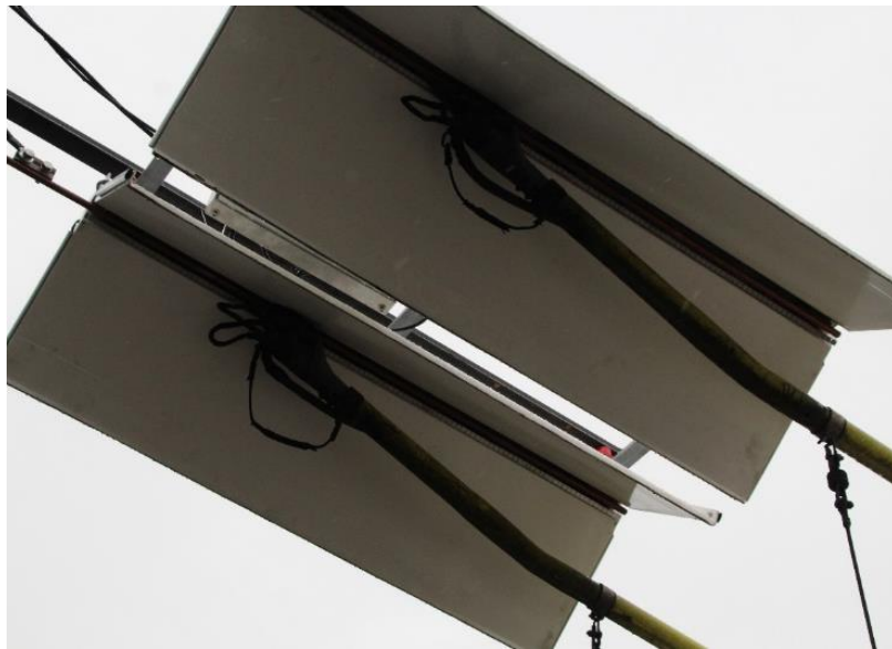
Fig. 5 – Fast charging connection point for trolleybuses, designed by the AREX company (Gdynia, Polen)
